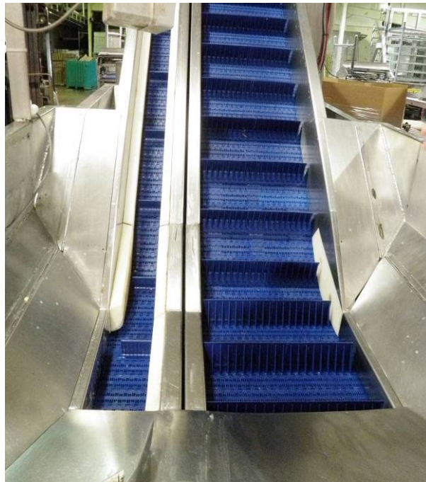
Figure 28. The dual conveyor belt picks up fish in small and large increments, to be used to fill the hoppers to the desired weight for packaging.
