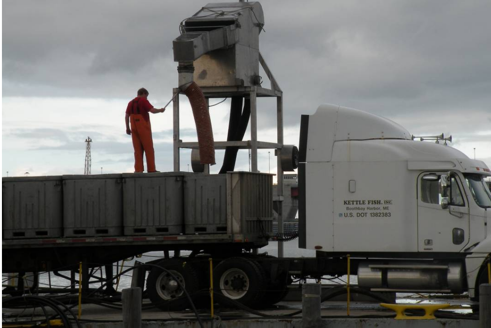
Figure 15. A flatbed truck carrying bait containers as it is being filled from the de-watering box. A man holds a tube in place to direct the flow of herring.
