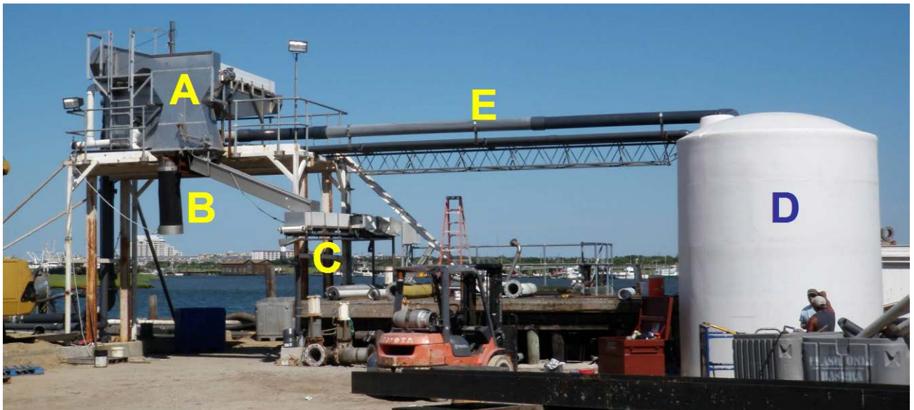
Figure 23. The herring, after pumped off the boat and to the de-watering box (A) are then are either deposited into trucks or poultry bins via a hose for bait sales (B) or into the facility via a conveyor belt (C) and then into tubes into the plant for the food market. Meanwhile cold water is re-circulated between the boat and the storage tank (D) via pipes (E).
