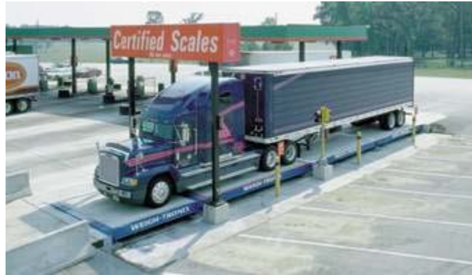
Figure 34. A truck scale in use (photo credit: http://science.howstuffworks.com/question626.htm )
